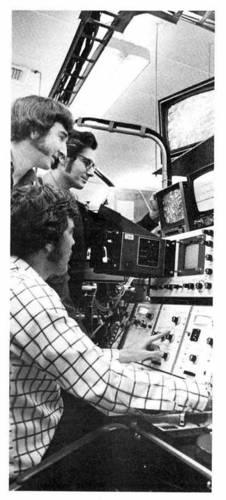
DETAILS OF DEVASTATION on a molecular level are seen when a material sample is subjected to CTR environment. Video system is connected to a scanning electron microscope focused on the target area of a 450 KeV positive ion accelerator. Researcher George Thomas (8334), upper right, Dan Morse (8334) and operator Les Brown (8313) conduct the experiment.
